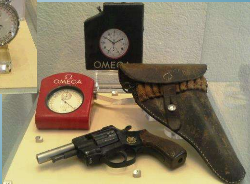
Case no 41 First interlinking sports timekeeping chronograph. Firing pistol will trigger the stopwatch start. The ending still manual
