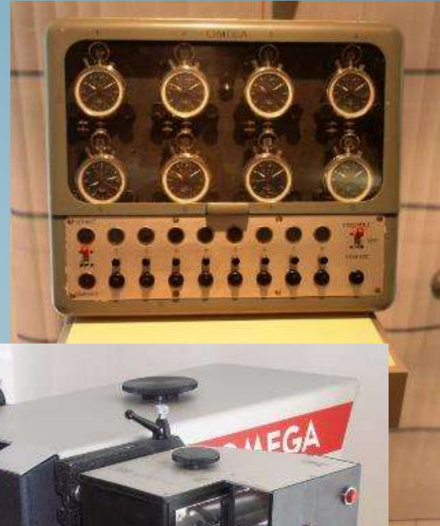
Robot timer that could follow timing of multiple athletes automatically
